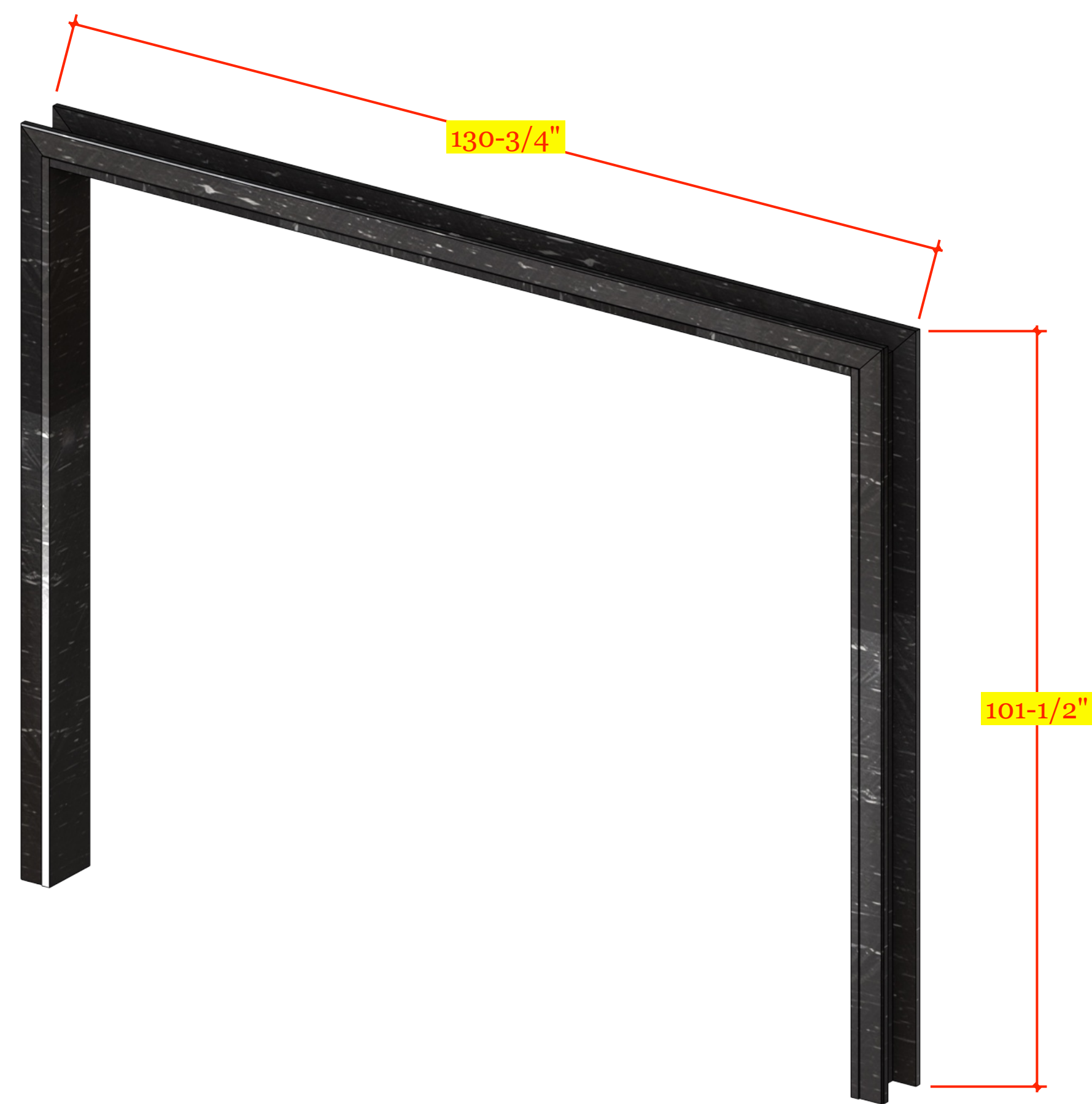
ISO A STONE JAMB AT DEN + CASING ISOMETRIC VIEW Scale: NO SCALE
